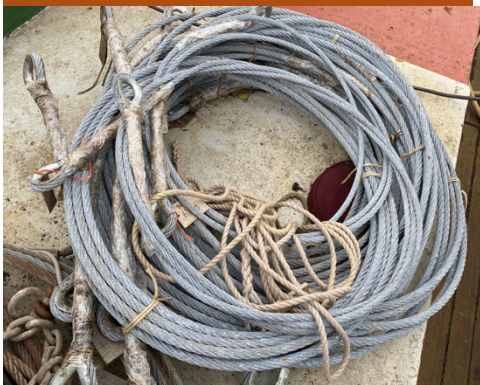
New steel rigging that has been 'hand spliced'! pending re-rigging in a few weeks
