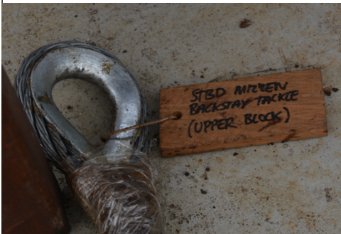
New steel rigging that has been 'hand spliced'! pending re-rigging in a few weeks
