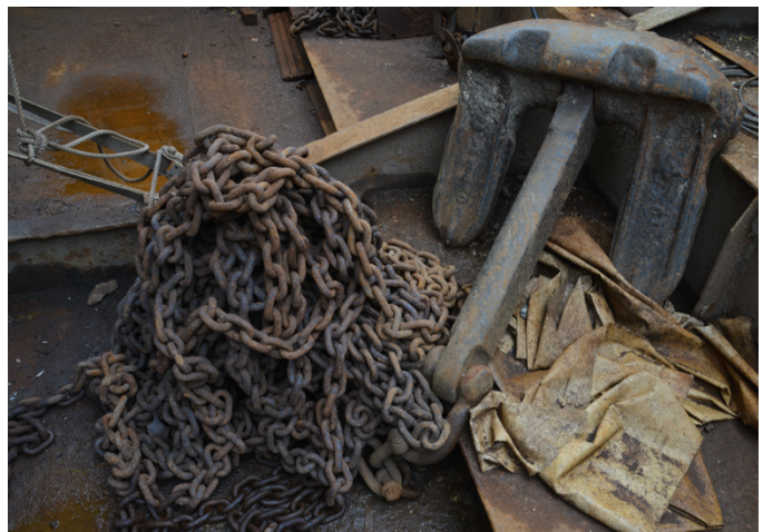
One of the main anchors (x2) removed to work on the chain lockers
